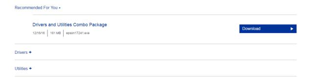
5. With the driver list open, download the Scanner Driver and Epson Scan 2 Utility. This is the TWAIN driver and the minimum needed to run the scanner.
